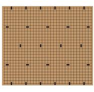
Recommended maximum stapling distance 15cm at edges and 20cm internally.
