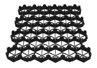
**TerraPave Porous Pavers** are an interlocking cellular paving system for ground reinforcement. The grids can be installed with either a grass or gravel filled surface and provide a durable, environmentally friendly reinforced surface able to cope with extremely heavy loads.
